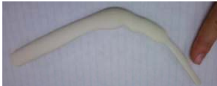
Figure 3.4: Plastic negative printed from rapid-prototyping machine
