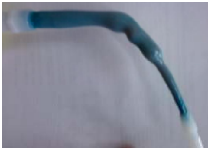
Figure 3.8: Primer-coated and glue-coated wax negative
