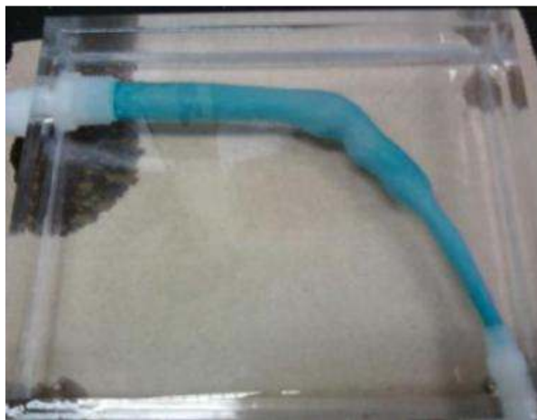
Figure 3.9: Wax negative casted in silicone
